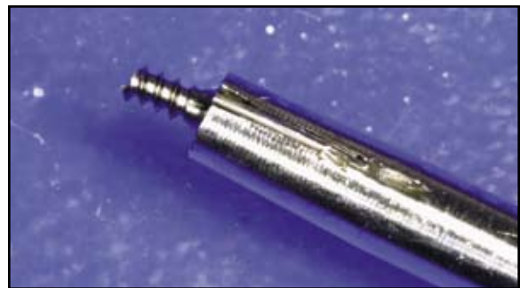
Fig. 6 Screw broken during insertion.
